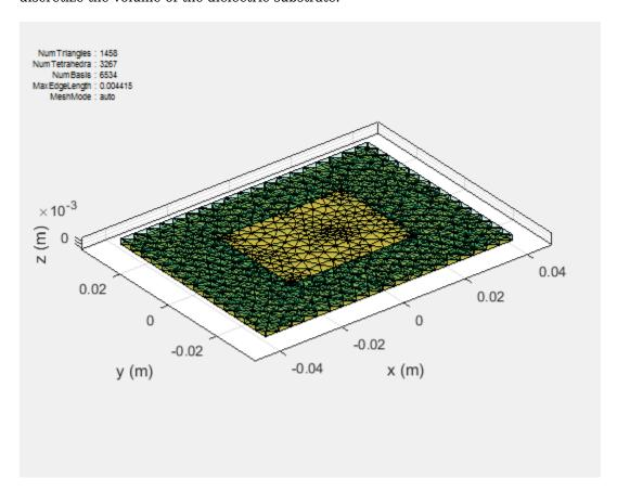
Thickness of the dielectric substrate is measured with respect to the wavelength. A dielectric substrate with thickness less than or equal to 1/50th of the wavelength is a thin substrate. When you mesh an antenna using dielectric in auto mode, thin substrates yield more accurate solutions.
