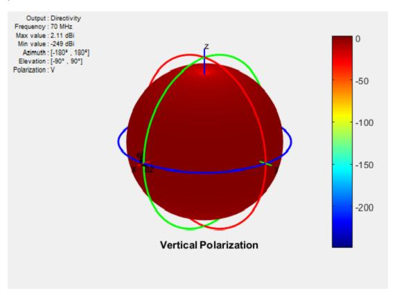
An AM radio broadcast antenna or an automobile whip antenna are some examples of vertically polarized antennas.
