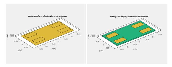
For example, the voltage vector matrix for a 2x2 array of rectangular patch antenna (with and without dielectric substrate) has four columns as each antenna can be excited separately.
