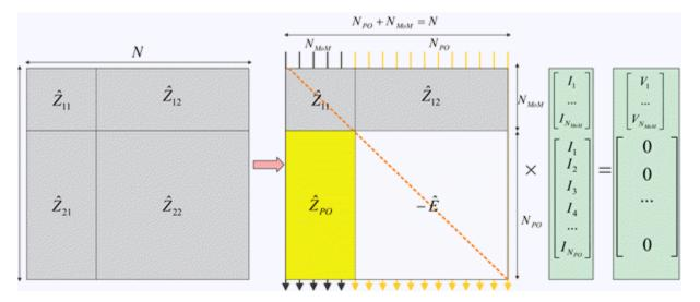
The figure shows the matrix interpretation of the hybrid MoM-PO solution and its comparison with plain MoM solution. The method assumes the antenna feeds gives the vector,  $\vec{V}$  that describes the excitation, which belongs to the MoM region only.
