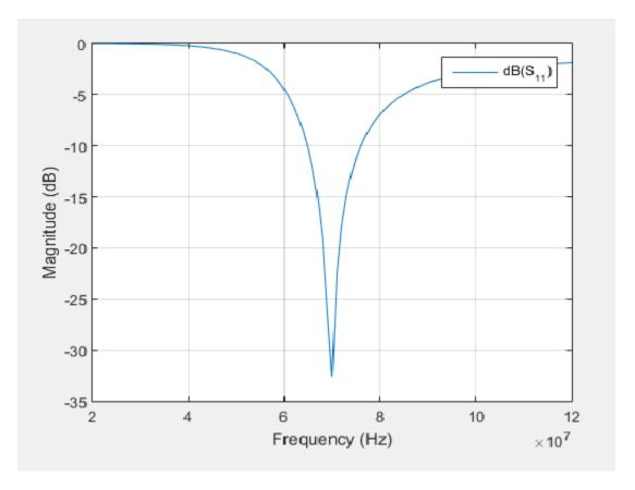
The reflection coefficient also gives the operating bandwidth of the antenna. Antenna bandwidth is usually the frequency band over which the magnitude of the reflection coefficient is below -10 dB.
