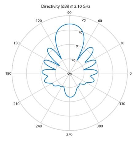
Half power beamwidth (HPBW) is the angular separation in which the magnitude of the radiation pattern decreases by 50% (or -3dB) from the peak of the main beam
