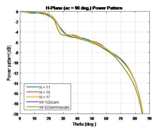
For finite arrays of size greater than  $10 \times 10$ , the scan element patterns in the E-, D-, and H-planes match the patterns of the infinite array scan element.
