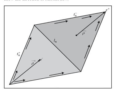
The basis function includes a pair of adjacent (not necessarily coplanar) triangles and resembles a small spatial dipole with linear current distribution. Each triangle is associated with a positive or negative charge.
