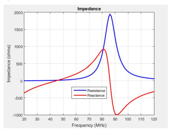
All the dimensions of this antenna are same as the monopole. The first resonance of the antenna is approximately  $45~\mathrm{MHz}$ . To view the accumulated charges on the top-hat monopole, use the charge function:
